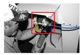
3. Place the recirculating tank under booth. (Make sure to remove all brushes, implements and hoses from inside box), place the draw hose end from the mounted pump into the slot provided.
